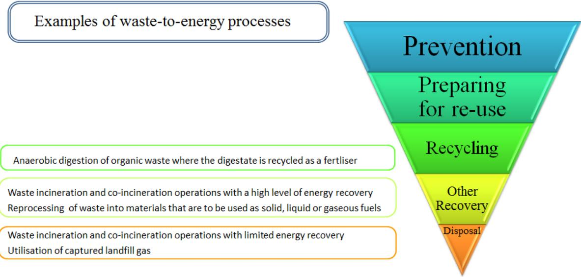
**Figure 1. The waste hierarchy and waste-to-energy processes**
